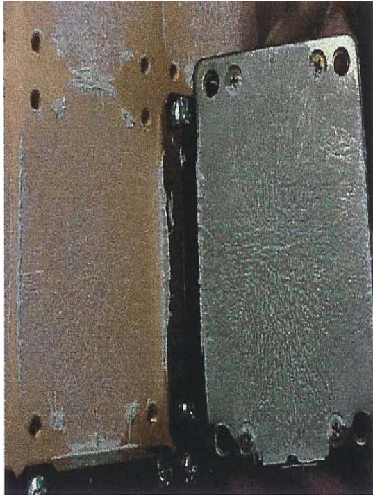
Poor distribution. Grease dried out.
